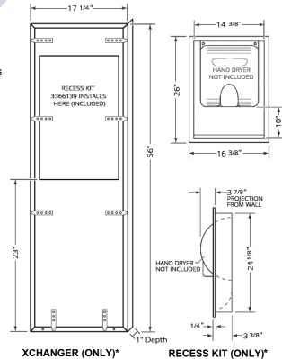
FBoth the XChanger (ADA Height) and Recess Kit 3366139 are included with Combo Kit 3366134
